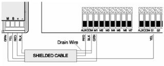
\* Connect drain wire to the COM terminal of PC4936 OR the black terminal of the station - NOT BO
